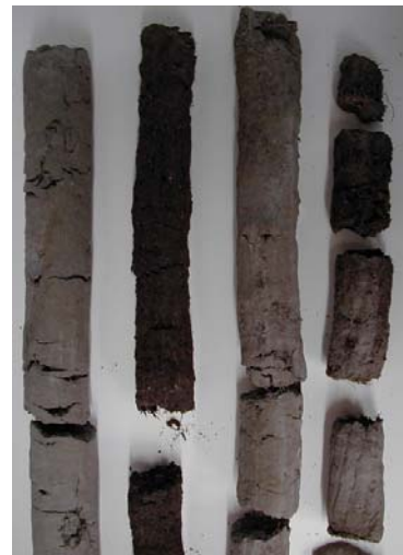
The cores from Willow Lake pictured above are 2.5” in diameter and 18” to 20” long.
